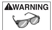
Operating this compressor can propel objects into the air, causing immediate eye damage. To protect yourself, always wear American National Standards Institute (ANSI) approved safety glasses or goggles when operating this equipment.
